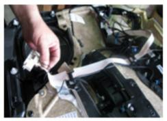
4. To plug and connect the power of the new mirror cover with arrow type light and manner light. Reinstall the new mirror cover with arrow type indicator as pictures G, H, I. onto the car with the main mirror component as picture J, K, L, M. Now it is installed completion (see picture N.). Please bottom the warning switch before to plug and connect the power of the indicator and manner light.
